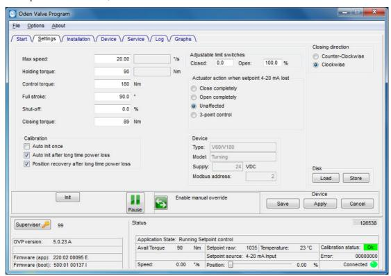
Check Firmware (app) and Firmware (boot), are like in picture, when using V5.0.23A program.
