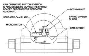
Total accessibility and simplicity provide rapid switch adjustment, once the lid and indicator dome are removed. The cam carrying sliders are spring loaded on splines, with the thumbscrew loosened the cam can be adjusted in seconds simply by lifting the slider and relocating it as required, re-tightening of the thumbscrew locks the slider in position and eliminates any possibility of creep.
