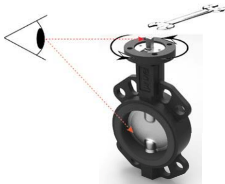
Figure 9 Valve handle removal
